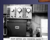
Sodium sampling flow and pressure controls
