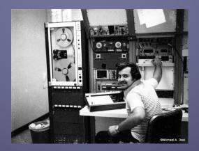
Data reduction using state-of-theart HP Analyzers and plotters
