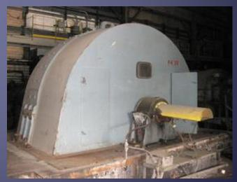
**GE 5000 HP DC Motor in steel mill** driving stainless strips across rollers
