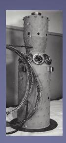
inch diameter prototype Low NOx
