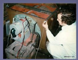
Motor housing vibration tests
